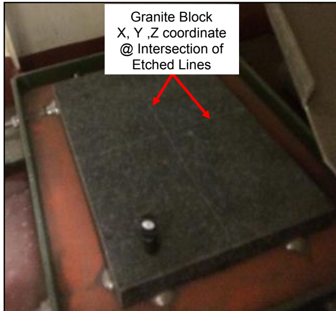
Fig. 2 – Granite Block located in Fwd Closet of C05 Stateroom Lounge
