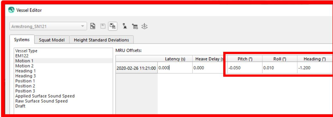
The screenshot shows the Vessel Editor interface for vessel Armstrong\_SN121. The 'Systems' tab is active, showing 'Squat Model' and 'Height Standard Deviations'. The 'MRU Offsets' table is highlighted with a red box, showing the following data:
