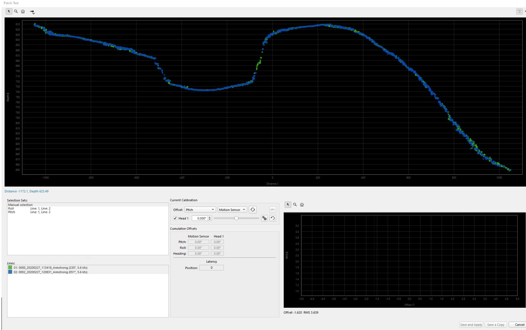
Calibration lines shown in the Qimera Patch Test Tool
