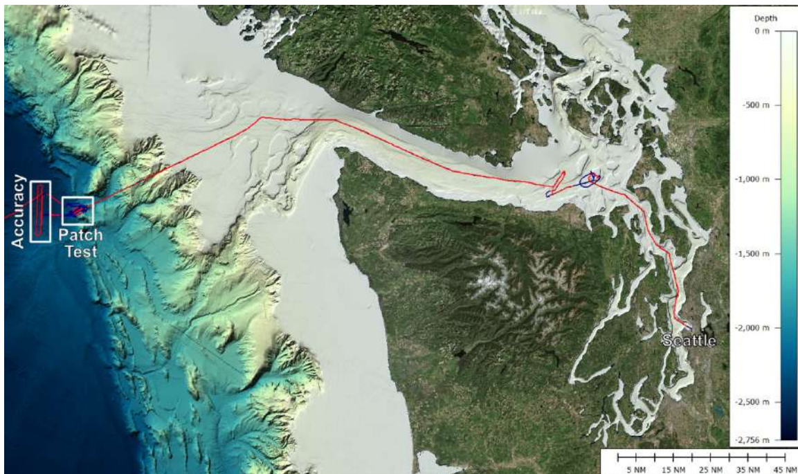
Figure 1. Calibration and accuracy testing sites in the Strait of Juan de Fuca and off the coast of Washington during HE17TA. These sites were selected based on availability of suitable seafloor features in the intended operational depth range for the EM122 multibeam echosounder. Swath coverage (acoustic extinction) data were collected up and down the slope in addition to over these test sites (red ship track).
